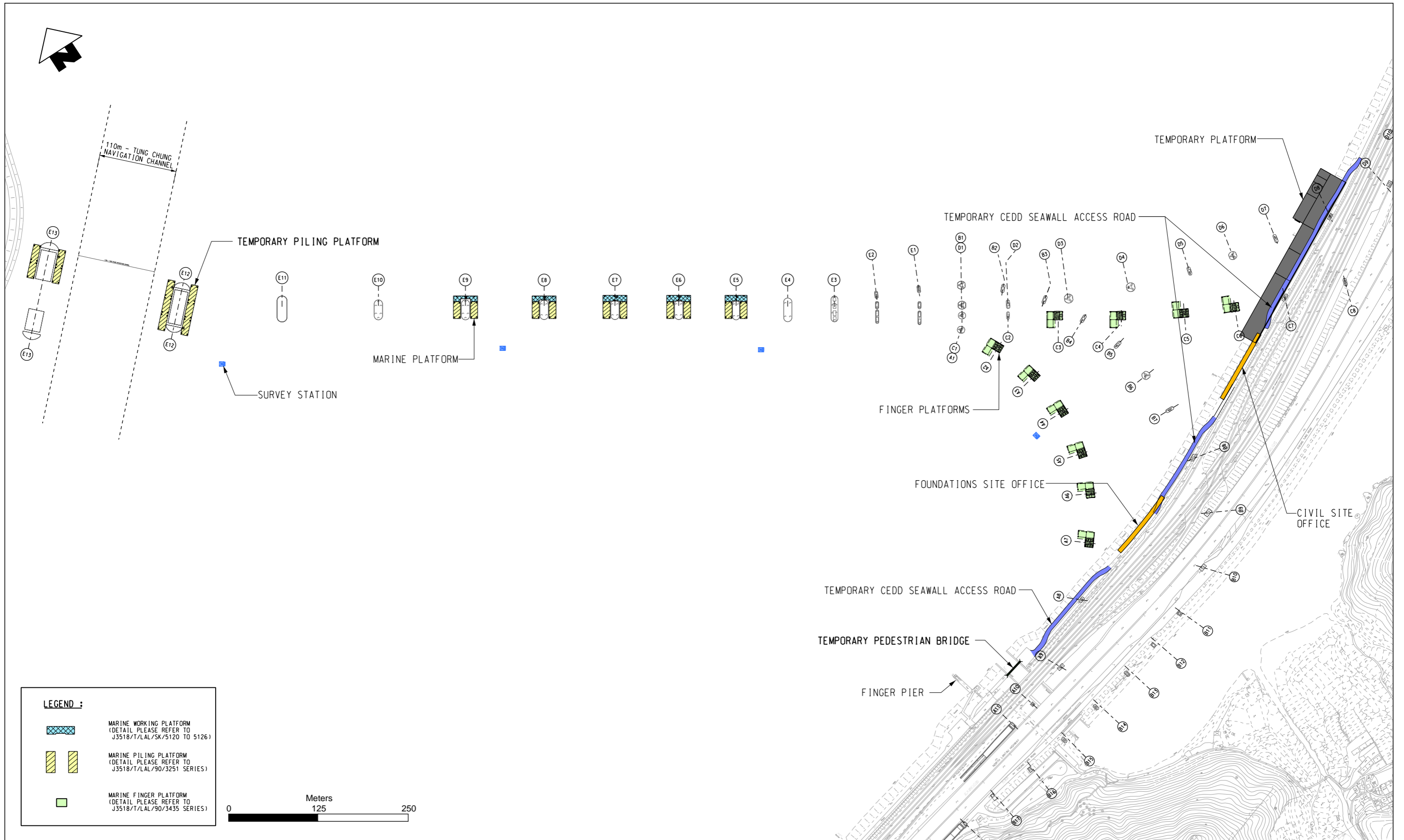
Figure 2.5 Construction Stages of Temporary Staging Platforms – Stage 4
