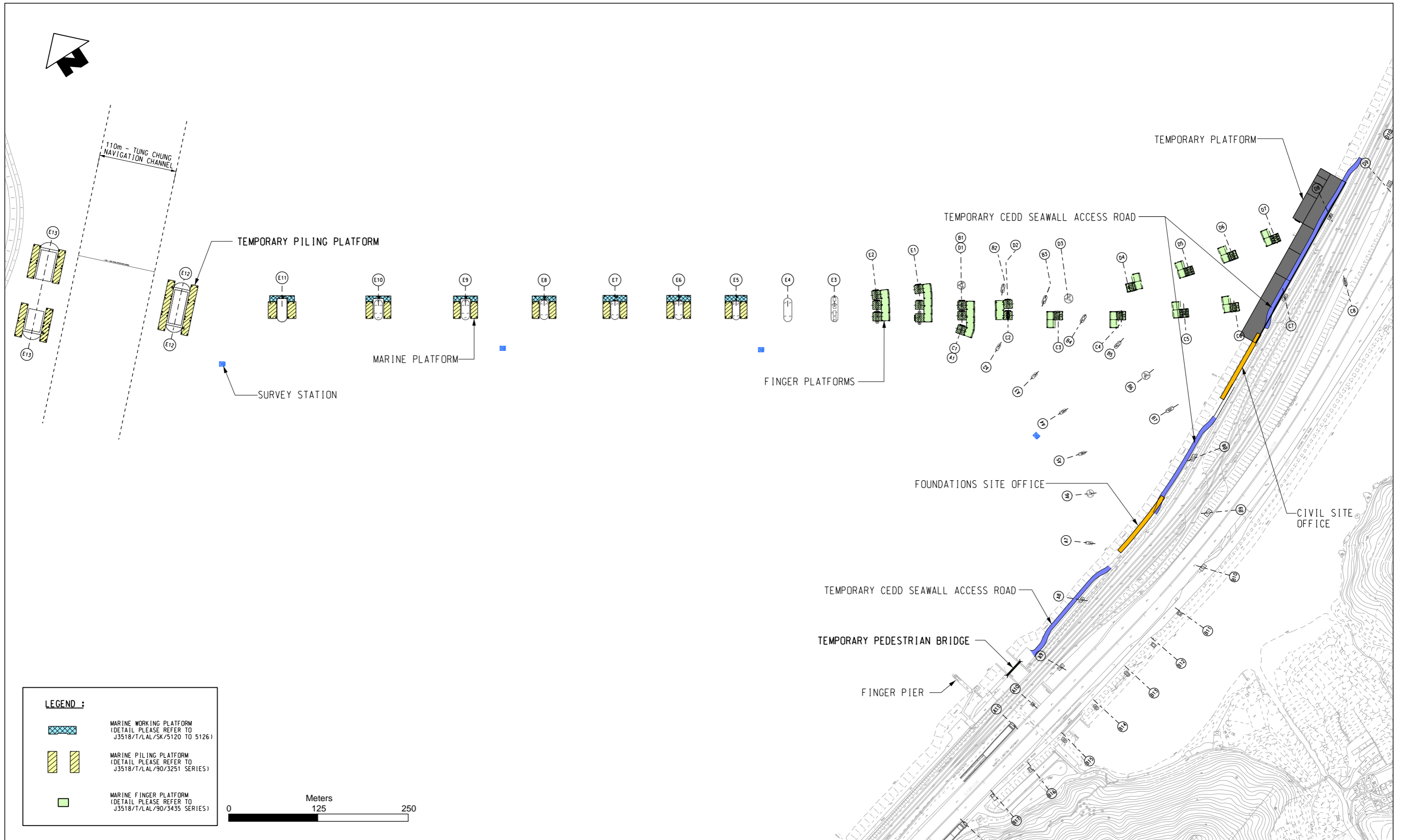
Figure 2.4 Construction Stages of Temporary Staging Platforms – Stage 3
