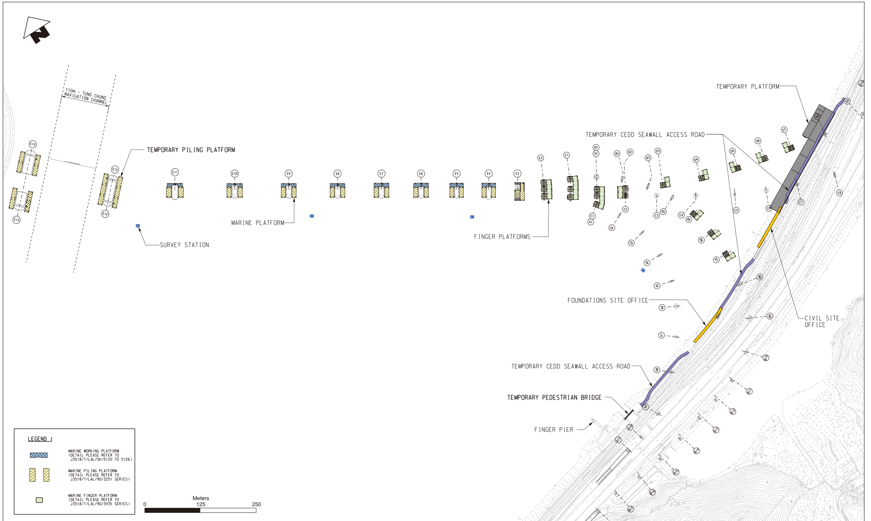
Figure 2.3 Construction Stages of Temporary Staging Platforms – Stage 2
