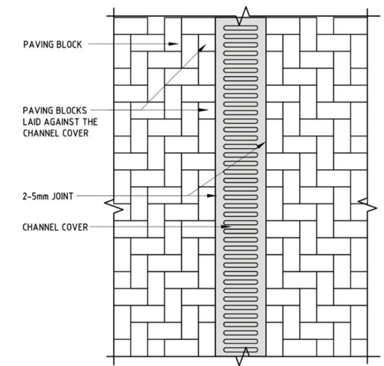
TREATMENT TO PAVING UNITS ADJOINING CHANNELS EDGES
